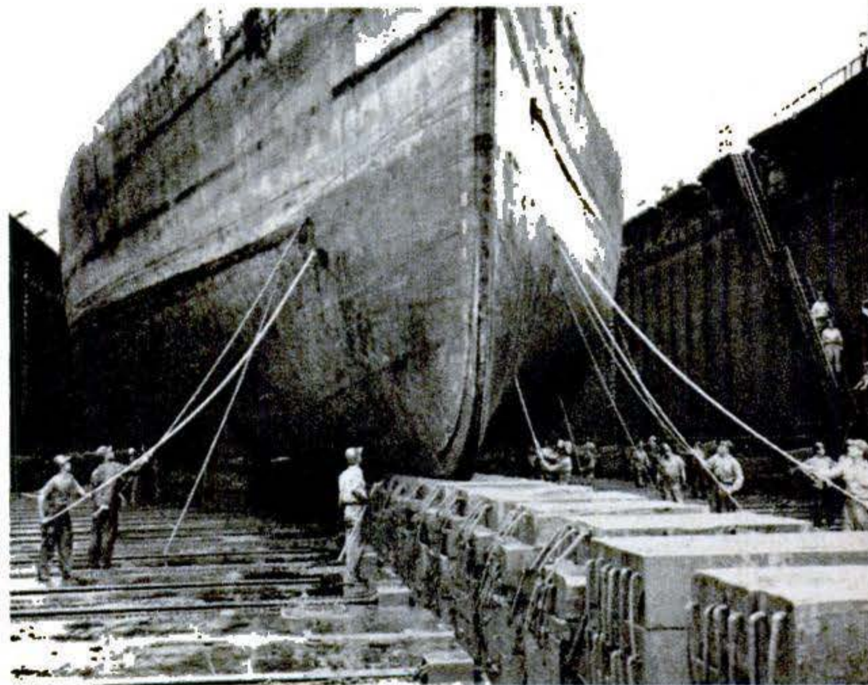
6. An overhauling crew swarms into dock as last of water drains out, leaving ship high and dry on the blocks. Using long-handled scrapers and wire brushes, men remove all traces of rust and marine growth from ship's bottom in preparation for repainting job.
